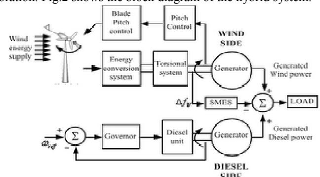
Fig. 2 Block diagram of wind-diesel hybrid power system
